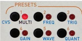
Each of the six CV inputs can be reassigned to one of 14 total modulation destinations. Available are six individual-channel and eight **Hex** modulation destinations. The six individual-channel destinations effect one user-assigned channel, while the eight **Hex** modulation destinations effect all six channels by modulating the parameters of the Hex macro control layer.
