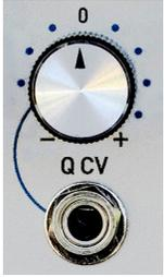
The **Q CV** input is an exponential control voltage input that is modified by its associated attenuverter and then summed with the value of the **Filter Q** control and the **6dB/V** input to determine the final resonance.
