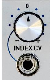
The **Index CV** input is a control voltage input that is modified by its associated attenuverter and then summed with the value of the **Mod Index** control to determine the final modulation index.
