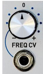
The **Freq CV** input is an exponential control voltage input that is modified by its associated attenuverter and then summed with the value of the **Filter Freq** control and the **1V/OCT** input to determine the final frequency.
