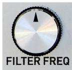
This control lets you set the filter's initial frequency over a range of 20Hz to 20kHz.
