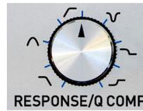
When both **Response Enable** controls are off, the **Response/Q Comp** control sets the amount of level compensation for the current Q.
