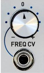
The **Freq CV** input is an exponential control voltage input that is modified by its associated attenuverter and then summed with the value of the **Osc Freq** control to determine the final **Mod Oscillator** frequency.
