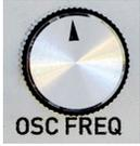
This control lets you set the **Modulation Oscillator's** initial frequency over a range of 20Hz to 20kHz.
