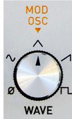
This control selects the output wave of the internal **Mod Oscillator**. It is continuously variable from Off through Sine, Triangle, Sawtooth and Square. As you move the control from Off to Sine, the sine wave will smoothly fade in. As you continue turning the knob, the output will smoothly morph between the adjacent waves.
