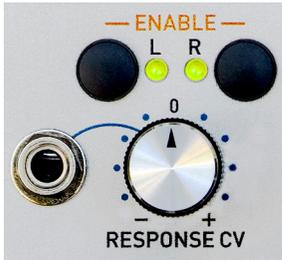
The **Response CV** input is a control voltage input that is modified by its associated attenuverter and then summed with the value of the **Response**
