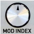
The **Mod Index** is a linear control that sets the initial value of the internal **Linear Mod Index VCA** that defines the degree to which the sum of the output of the internal
