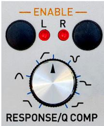
When one or both of the **Response Enable** LEDs are on, this control lets you select the initial filter response characteristic for one or both of the two channels.
