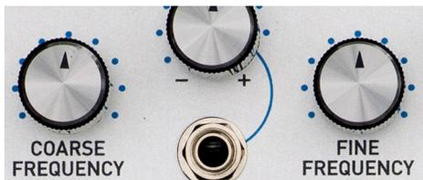
Using the COARSE FREQUENCY and FINE FREQUENCY controls, the Carrier Oscillator's initial frequency can be set between 20Hz and 20kHz.
