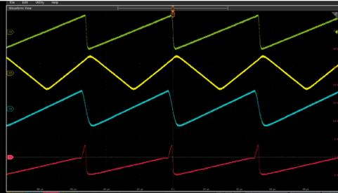
Finally, I realized that I've never seen anybody play with the phase relationship between hard synced oscillators. Combining that with Zing modulation gives even more voltage controlled timbral variation. These waveforms differ only by the phase of the MOD 2 oscillator!
