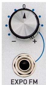
The EXPO FM Input is a control voltage input that is modified by its associated attenuverter and then summed with the value of the Coarse and Fine Frequency controls and the 1V/OCT input.
