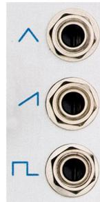
The Carrier Oscillator provides simultaneous triangle, sawtooth and pulse outputs.
