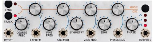
Varies the phase of the Mod 2 Oscillator compared to the Carrier when Mod 2 Sync is enabled. Modulates it via the CV input through an attenuverter.
