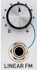
The LINEAR FM Input is an AC coupled control voltage input that is modified by its associated attenuator to allow Linear Frequency Modulation of Trident's output frequency.
