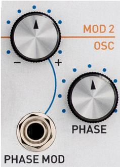
Modulation Oscillator 2 is identical to Modulation Oscillator 1, with the exception that it provides an additional CV controlled parameter: Modulation Phase.
