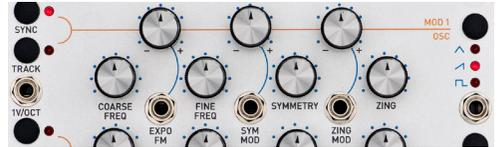
Sets the amount of a Mod Oscillator's Zing modulation of the Carrier Oscillator. Modulates the Zing amount via the CV input through an attenuverter.
