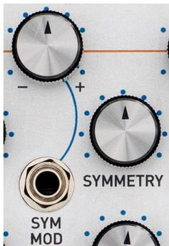
The SYMMETRY control lets you smoothly and continuously vary the shapes of the Mod Oscillator's waveforms. The effect on the various waveforms are as follows:
