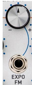
The EXPO FM Input is a control voltage input that is modified by its associated attenuverter and then summed with the value of the Coarse and Fine Frequency controls and the 1V/OCT input. As above, when the Track function is active, it is also summed with the Carrier Oscillator's COARSE and FINE FREQUENCY controls, 1V/OCT input, and EXPO FM input.
