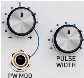
The PULSE WIDTH control lets you set the initial pulse width of the Carrier Oscillator's pulse wave output from 0% to 100%.
