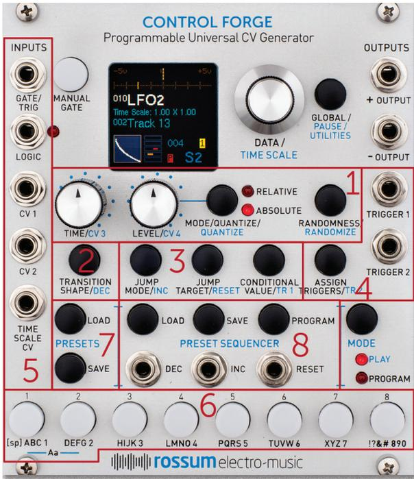
**1 TIME & LEVEL** Sets the duration and target level of each segment. Levels can be defined absolutely or relative to the ending level of the previous segment, can be quantized to the nearest 1/12 volt, and can have a range of randomness of either linear or gaussian distribution.
