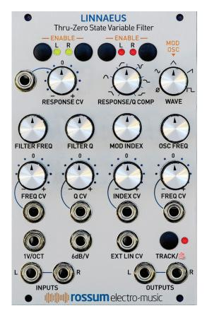
**FILTER FREQUENCY** Exponentially voltage-controllable from sub-audio to ultrasonic via precise 1V/OCT and attenuverted CV inputs.
