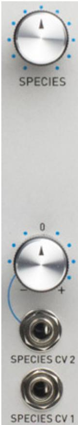
Evolution's Species section provides manual and CV control of the level of the signal into Evolution's distortion circuitry.
