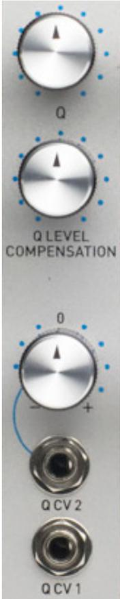
Evolution's Q section provides manual and CV control of the height of the resonant peak at (or near) Evolution's cutoff frequency, as well as the level of the frequencies below the resonant peak. (See the discussion of the effect of the Genus setting on the frequency of the resonant peak below.)
