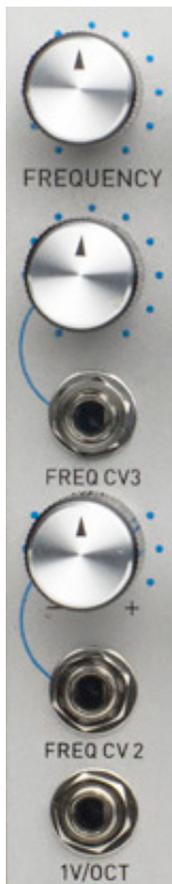
Evolution's Frequency section provides manual and CV control of Evolution's cutoff frequency (i.e., the frequency above which the amplitude of the signal is attenuated).
