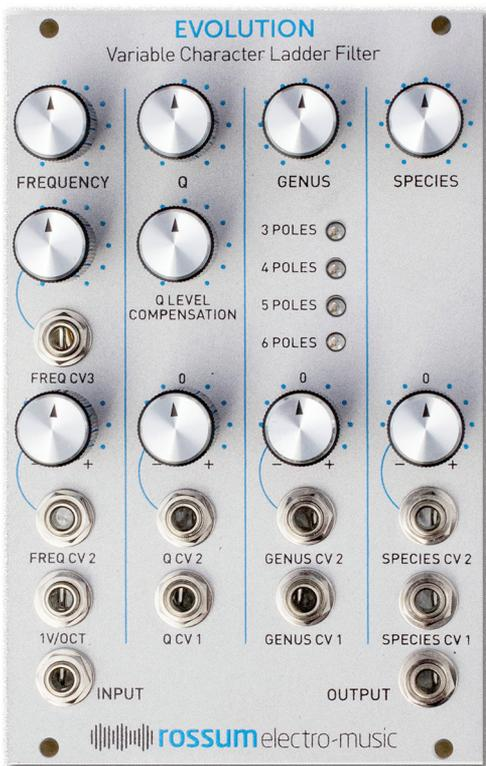
**FREQUENCY** Controls the initial cutoff frequency of the filter. The range (without CV input) is from approximately 20Hz to 20kHz when 4 poles are selected.
